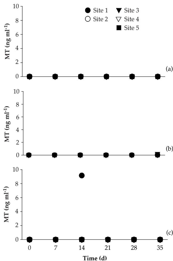
Figure 4. Concentration of 17 $\alpha$ -methyltestosterone (MT) in water from five sampling points (sites 1–5) measured at different times during masculinization Trial 2. Treatments were: (a) no activated charcoal (EU-1); (b) 2.5 kg of activated charcoal (EU-2); and (c) 5.0 kg of activated charcoal (EU-3). For this trial new mineral charcoal was used in the filtration systems.
