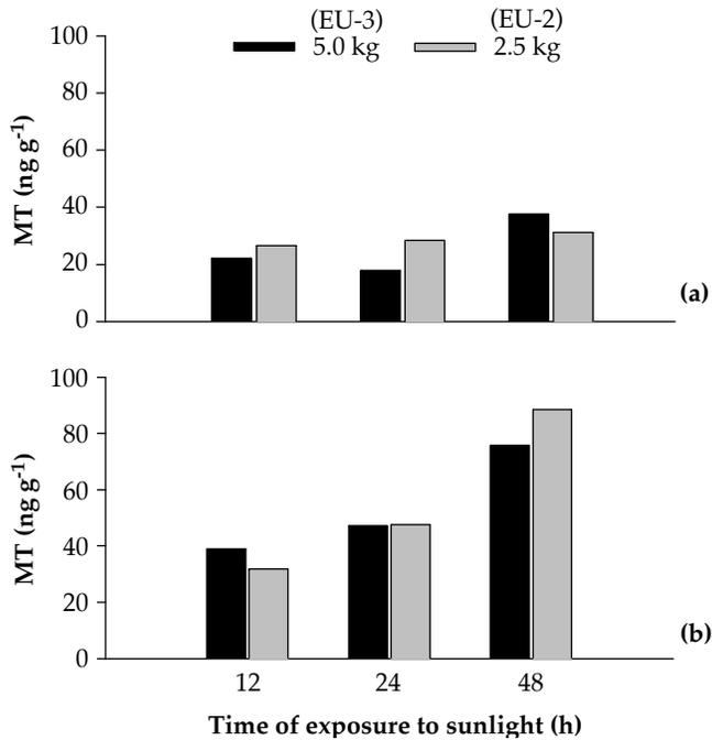
Figure 5.  $17\alpha$ -methyltestosterone (MT) concentrations in charcoal after being exposed to sunlight; (a) mineral charcoal used in Trial 2 and (b) vegetal charcoal used in Trial 3. Legend identifies the amount of charcoal used in each treatment.
