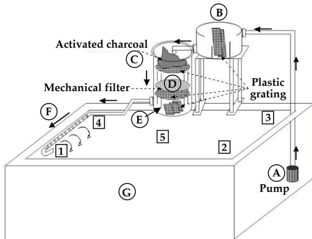
Figure 1. Intensive masculinization system adapted with a charcoal filter. Components are: A) submersible pump, B) sediment trap, C) charcoal filter section, D) mechanical filter section, E) biological filter section, F) return PVC pipe (creates a water curtain), and G) concrete tank ( $4.0 \times 1.8 \times 1.2$  m). Sampling points are indicated by numbers (1–5). Details are not drawn to scale.
