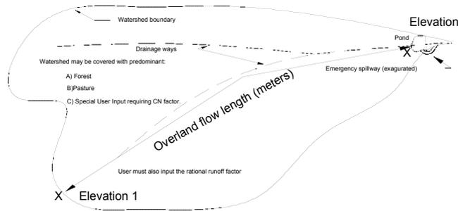
Figure 2. Schematic of watershed also showing the watershed pond.
