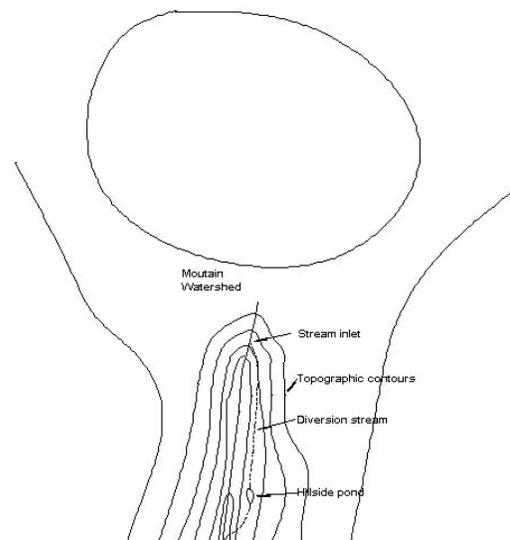
Figure 5. Hillside pond with stream diversion for general purpose water supply. Not shown are levee ponds being supplied at a more or less constant rate from the hillside pond.
