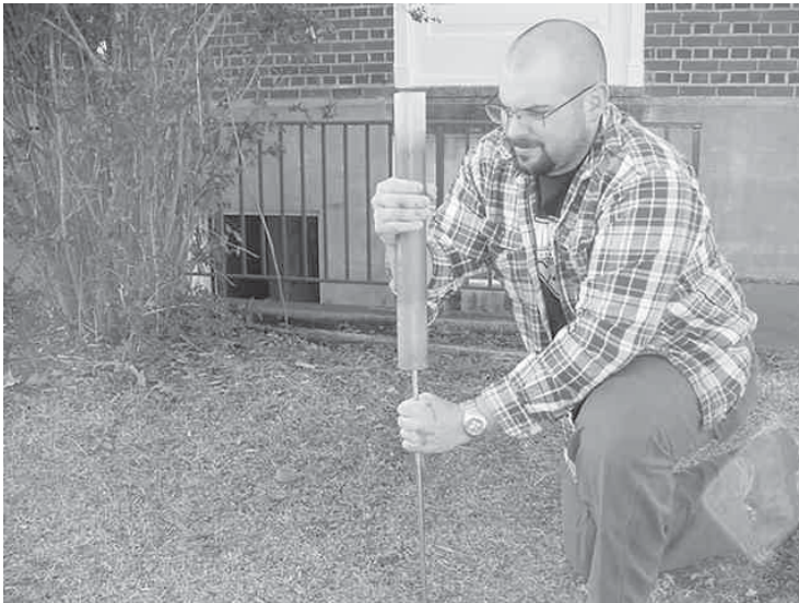
Figure 11. Use of plunger to push core from liner tube.
