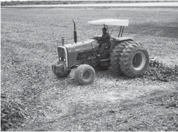
Figure 9. Tractor with extra wide tires to prevent rut forming during tillage of pond bottoms.
