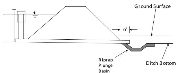
Figure 3. Cross-section of a pond embankment showing the drainage structure.
