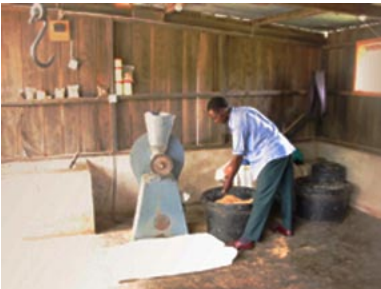
The pelleter resembles a meat mincer and is driven by a single phase 1.5 hp motor. It was developed in collaboration with the engineering company East African Foundry Works in Nairobi. The first of its kind to be made by local artisans, it has a capacity to produce approximately 30 kg pellets of feed per hour. J. Kariuki, Sagana, is pictured.
