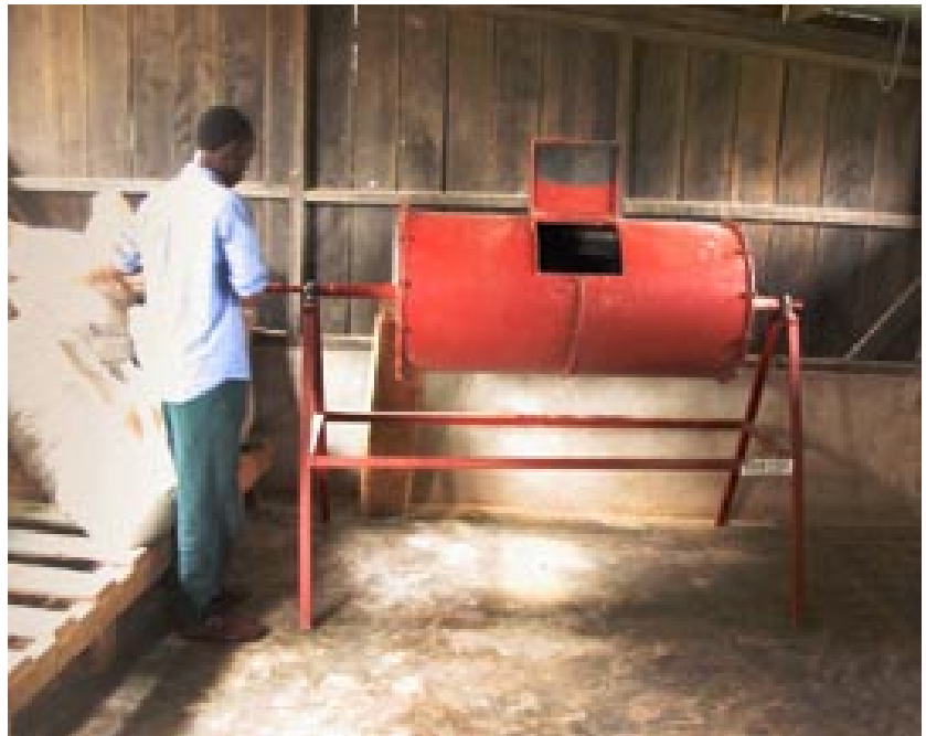
The mixer has a capacity of 1.5 m 3 and can mix 50 kg of feed at a time. It is manually driven by using a well designed handle. It can also be adapted to be operated by a gasoline engine or electrical power. J. Kariuki, Sagana, demonstrates.
